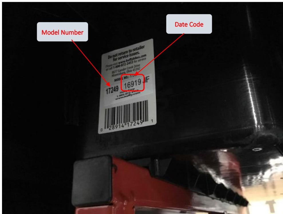
**Location of Model Number and Date Code – under wheel well on left rear side**
